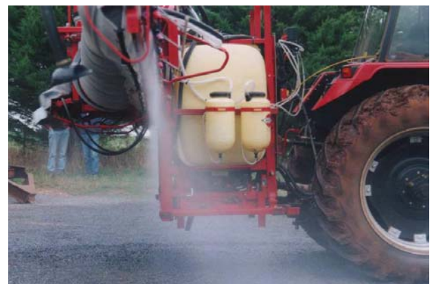
Photo1. Check sprayer and calibrate using water only.
